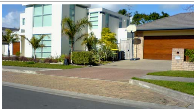
Formed on-road parking bays can be undermined by inconsiderate placement of vehicle driveways and garages. Lost parking bays cannot be easily replaced once the roadway has been formed.
